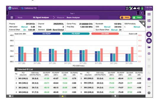
To achieve true beamforming, network technicians will need to identify the signal at beam level and test the performance of all the algorithms and handoffs, as well as validating the signal to interference ratio prior to service activation.
